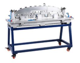
Front bumper lower trim panel checking fixture
