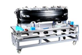
Rear protection checking fixture
