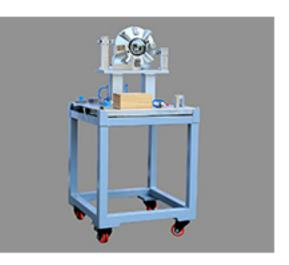
Fog lamp checking fixture
